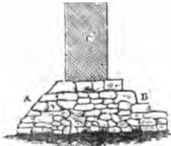
Fig. 27.—Section of foundation courses and superstructure. A, batter. B, offsets. C, superstructure.
